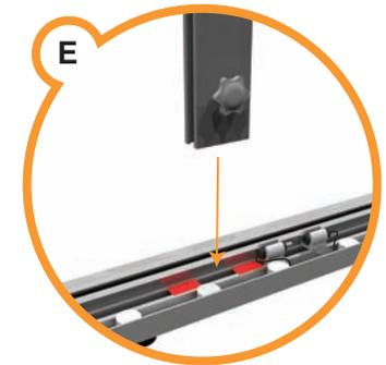
Locate the 'insert vertical here' sticker and secure the central column to the frame using the CBX connectors.
