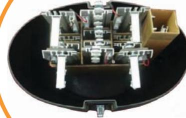
Insert the central extrusions A10-A12 into the box provided and position as pictured above.
