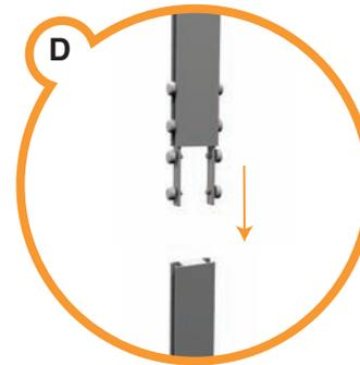
Slide the central support A11 onto A10 & A12 and tighten thumb screws.
